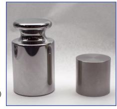
Figure 3: 1 kg of Stainless Steel compared with 1 kg of platinum-iridium
